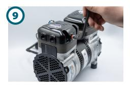
Carefully remove the fan guard with a screwdriver. Rotate the fan again to ensure the compressor rotates freely. Replace the fan guard.
