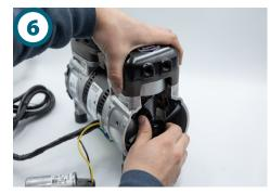
Place both attenuation chambers directly onto the top surface of the valve plate.
