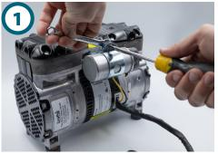
Using a flat head screw driver and a 8mm wrench, loosen the capacitor bracket. Once the bracket is loose, slide the capacitor out of the bracket and set it next to the compressor. **Do not remove the rubber cover, or wires connecting the capacitor to the compressor.**
