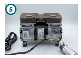
Place the new valve plate, with O-rings attached, directly onto the two cylinders and pump body.
