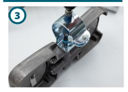
Using a 1/4" nut driver, remove the two screws holding the capacitor bracket to the valve plate. Remove the capacitor bracket. Set it and the two screws to the side
