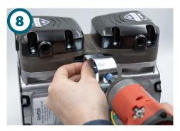
Using the two screws removed in step three, install the capacitor bracket on the new valve plate. Slide the capacitor into the bracket. Tighten the bracket around the capacitor using a flat head screw driver and the 8mm wrench to secure it in place
