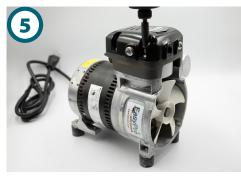
With the valve plate and attenuation chamber outer profile aligned, install the (4) 10-32 Torx screws (torque to 50 in-lbs.) in a star pattern.
