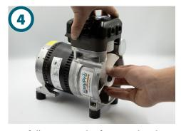
Carefully remove the fan guard with a screwdriver. Place the attenuation chamber directly onto the top surface of the valve plate.
