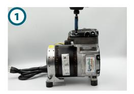
Unfasten all (4) existing 10-32 Torx button head screws. Remove and discard the original black head, valve plate, respective O-rings and screws. Do **NOT** displace the cylinders below the valve plate. Keep secured in body and rod.
