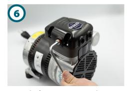
Rotate the fan again to ensure the compressor rotates freely. Replace the fan guard.
