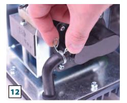
Reattach L-tube and secure with existing pinch clamp.
