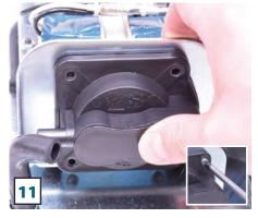
To install new diaphragm outlet cover, be sure to properly align holes and hold tightly while securing with screws. Gradually tighten screws around the assembly until evenly tight to unit.
