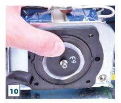
Secure diaphragm to magnet with new washer and nut. Push the magnet from behind to help tighten the nut to the magnet. Be sure to get tight. A drop of Blue/Removable Loctite<sup>®</sup> may be used.
