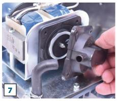
Remove diaphragm frame, may need flat head screw driver to separate from unit - note orientation for proper installation of new one (step 8).
