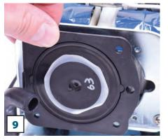
Line up new diaphragm to match how old one came off. Match up to notch on motor housing.
