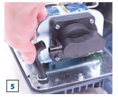
Repair one side at a time. Slide pinch clamp down the L-tube and remove top of L-tube from diaphragm outlet.
