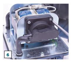
Remove the four screws from the plastic diaphragm housing with #2 Phillips screwdriver.
