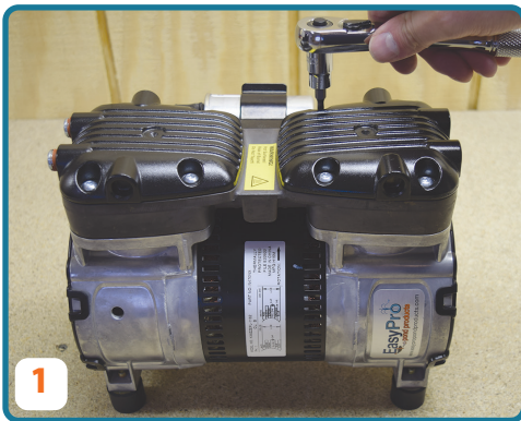
1 Remove screws from the head of compressor using T25 Torx driver. Remove the head.
