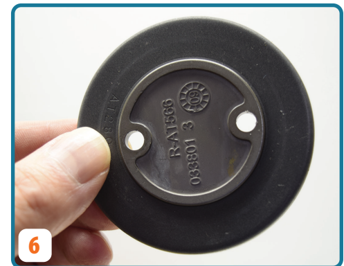
6 Remove new piston cup(s) from protective cardboard packaging. Set new piston cups onto retainer plate, these parts will sit flat against each other.
