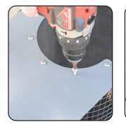
1. Position the support as shown and screw it to the bottom of intake screen. **Be careful to not over tighten.**
