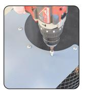
1. Position the support as shown and screw it to the bottom of intake screen. **Be careful to not over tighten.**
