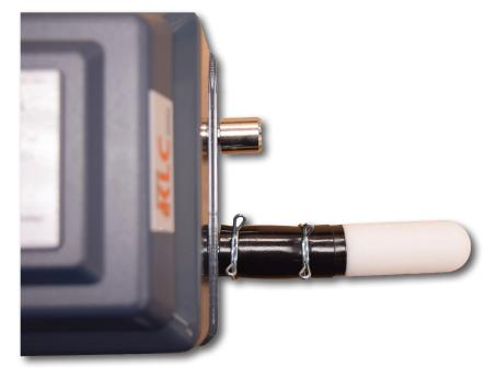
Install the air inlet filter as shown. Be sure to install on the inlet side only. See bottom of unit for identification.
