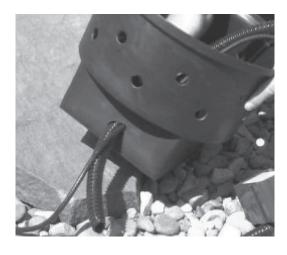
Slide tubing through big hole in base of filter. Use 1/2" to 1" tubing.
