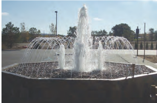
Nozzles can be installed vertically or at an angle. This feature has smooth jet nozzles surrounding frothy nozzles.
