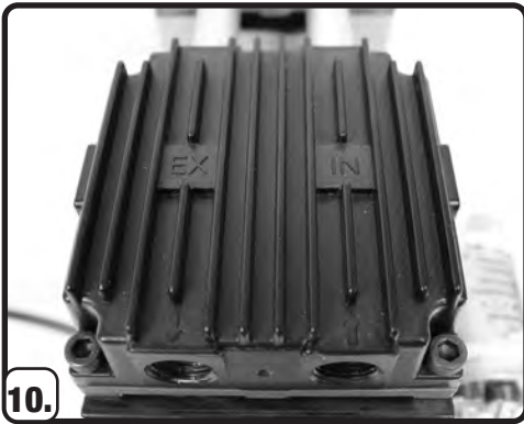
10. Replace the head of the compressor ensuring the correct, original orientation.
