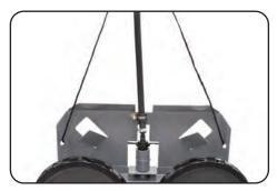
Use rope looped through holes in base to assist lowering assembly to pond bottom. Carry only by base, do not lift by diffusers.
