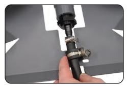
Fit padded hose clamp over tubing. (Use 17.5mm clamp for <sup>3</sup>/<sub>8</sub>" tubing or 25.5mm clamp for <sup>1</sup>/<sub>2</sub>" and <sup>5</sup>/<sub>8</sub>" tubing)
