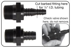
1. <sup>3</sup>/<sub>4</sub>" MPT barbed check valve is designed to be used with <sup>1</sup>/<sub>2</sub>" or <sup>3</sup>/<sub>8</sub>" I.D. tubing. Use larger barbed fitting for <sup>5</sup>/<sub>8</sub>" ID tubing
