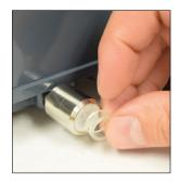
Install retainer ring to hold filter into place.
