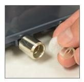
Remove old filter elements from compressor. These can be saved and cleaned if in adequate condition. Pinch clamps and connecting tube will be re-used.
