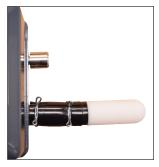
Install the air inlet filter as shown. Be sure to install on the inlet side only.
