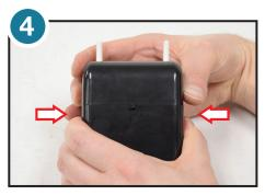
4. To remove the housing cover, squeeze the back section while alternately squeezing and pulling the front section off. Use a flat screw driver with a twisting motion (avoid prying) to loosen front cover and then pull front section off.
