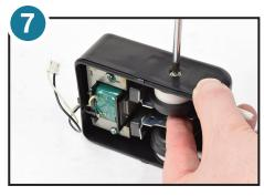
Remove screws from side of internal housing to remove diaphragm assemblies from unit. Inspect magnets and clean if needed.
