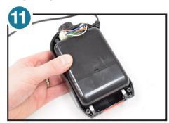
Reinstall outlet bushings and place internal housing into base. Reconnect electrical connection.
