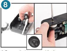
Remove diaphragm assemblies from unit. Remove the black seals shown in the inset photo and press them into the sides of the new diaphragm assemblies. Install new diaphragm assembly by holding it securely to the side while tightening screw.
