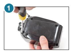
1. Unplug unit and remove four screws from bottom of main housing.
