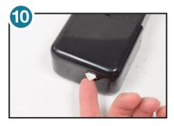
Guide electrical connection through the hole in back housing cover and reinstall front cover.
