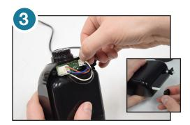
Carefully disconnect the electrical connector. This will be the connector with the black and white wires. Once disconnected the internal housing section can be removed. Remove outlet bushings.
