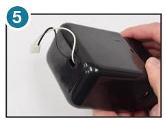
Remove the back cover section while carefully guiding the electrical connector through the rectangular hole.
