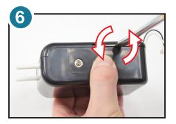
To remove lid of internal housing, squeeze longer sides tightly to create a small space for a flat screw driver. Use a slight twisting motion with the screw driver to release the lid of the internal housing.
