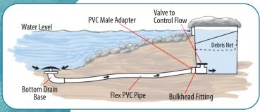
The bottom drain should be placed at the deepest part of the pond with the tubing running under the liner to the skimmer box.
