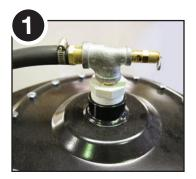
Loosen the clamp on the heater hose on top of the compressor and remove it from the brass hose barb.
