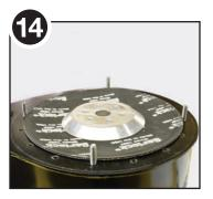
Place four short threaded alignment studs in compressor top; one each at front, back, left and right. Like the face of a clock, it would be at 12, 6, 3 and 9 o'clock positions. Rotate shaft so piston is at the bottom of its stroke. This pulls diaphragm away for securing the lid.
