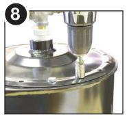
Remove compressor lid by removing the 16 bolts on the top of the lid with 1/2" socket wrench or driver. You will now have access to larger aluminum valve retainer and diaphragm.
