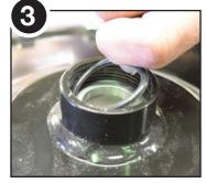
Remove the upper o-ring, the aluminum valve retainer and lower o-ring from compressor top. Be sure to note the orientation of the aluminum valve retainer as it will need to be re-installed in same way
