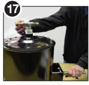
To check if there is pressure being created, turn the compressor shaft while holding your thumb on the end of the brass hose barb. If you have pressure, reconnect the heater hose and put compressor back into service on the windmill.
