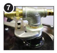
Reinstall the outlet plumbing assembly to compressor top. Be sure not to cross thread or over tighten.
