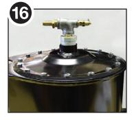
Carefully rotate the compressor shaft so that the piston is at the top of its stroke. If valve retainer comes in contact with the underside of the lid, you may have an alignment issue and should contact your Becker Windmill Dealer or EasyPro Pond Products for assistance.
