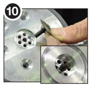
Remove the old rubber umbrella valve and install new one. It is not necessary to cut off the stem this time.
