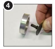
Remove the rubber umbrella valve from the aluminum valve retainer and install new umbrella valve. It may help to wet the valve stem slightly.
