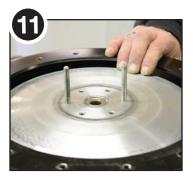
Remove the old diaphragm. Install long threaded studs in push plate as shown to help align diaphragm and aluminum valve retainer. They are temporary items and will be removed for final reassembly.
