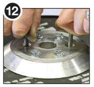
Place new diaphragm and reinstall aluminum valve retainer over alignment studs. Start four screws to maintain alignment and remove threaded studs for last two screws.
