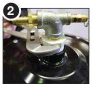
Remove the outlet plumbing assembly at the white bushing from the compressor top.
