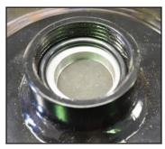
Place one o-ring into the threaded section on top of lid. Next install aluminum valve retainer and second o-ring on top of valve retainer. Be sure each item is properly seated and the valve retainer is in the correct orientation.
