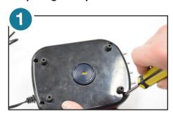
1. Unplug unit and remove four screws from bottom housing.
