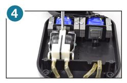
4. Remove diaphragm assemblies leaving air tubes. Inspect magnets and clean if needed.
