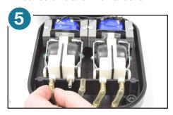
5. Install new diaphragms, reuse metal bracket to secure to base with screw and reattached air tubes.
