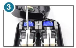
Remove screws that hold diaphragm assembly to base. Keep metal bracket at back.
