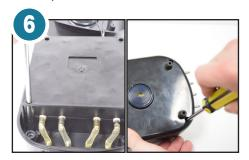
6. Reinstall internal cover and bottom housing with corresponding screws.
