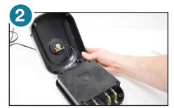
2. Carefully lift top back to have access to internal cover. Remove four screws and internal cover.
