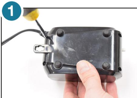
1. Unplug unit and remove four screws from bottom housing.
