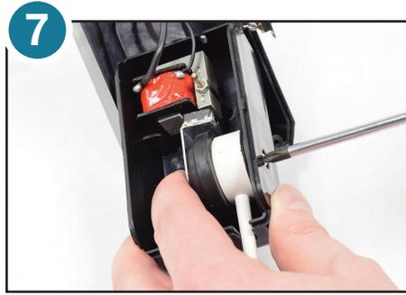
7. Press the black seal into the side of the new diaphragm assembly. Install new diaphragm assembly by holding it securely to the side while tightening screw.
