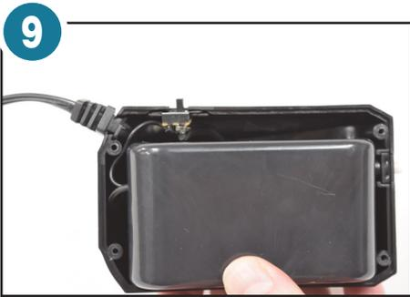
9. Place internal housing back into top of main housing. Arrange cords and switch to avoid pinching when reassembling main housing.
