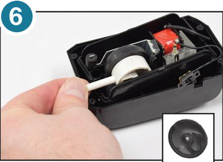
6. Remove diaphragm assembly from unit. Inspect magnets and clean if needed. Remove and save the black seal shown in the inset photo. This is not included in this repair kit. You will use this in step 7.
