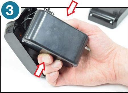
3. To remove lid of internal housing, lift internal housing without straining electrical cords, squeeze longer sides tightly to create a small space where a flat screw driver can be placed.
