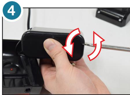
4. Instead of prying, use a slight twisting motion with the screw driver to release the lid of the internal housing.
