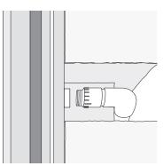
Determine the placement of additional fittings (elbows, tees, and extra pipe). Cut and glue all the pieces together to fit the application.
