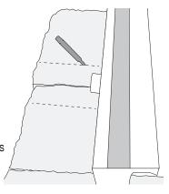
If the lighting option is purchased the LED light strip can be fitted into the back of the spillway. There are brackets on the ends of the light bars with holes in them. These brackets are for other applications. The LED light bar should fit snuggly into the back of the spillway. If necessary, a small amount of silicone can be used as an
