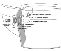
1 1 Before installing the float switch auto fill, loosen the Phillips screw to place float in proper orientation. It may be necessary to remove the screw and move the brass arm which holds the float to the
