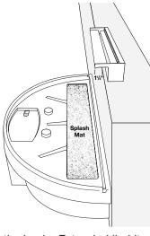
x 39" splash mat included with the basin. Extended lip kits come with 14" x 39" additional splash mat to be installed on top of basin (see page one).
