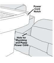
Once the spillway placement has been determined in the block wall, the block will need to be cut to allow for the plumbing connections on the back of the spillway. Use appropriate tools and extreme care when cutting block. Consult block manufacturer recommendations for properly cutting block being used.
