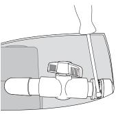
assembly is installed onto the pump, carefully lower the pump and assembly into the pump chamber. Line up the pump discharge with the pre-installed fitting. Again ensure that the pre-installed fitting is tight. Connect the pump discharge to the pre-installed fitting with the rubber coupler. A nut driver or screwdriver should be used to tighten the clamps. Ensure that both clamps are tight.
