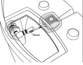
side as shown. This will allow for easier adjustment of the float to proper water level. Then thread the float switch assembly into the reducer bushing. Adjust the brass rod and float to approximate level of desired water level. Final adjustment should be made when final water level is determined.
