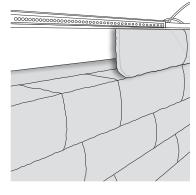
weight bearing support. Consult a qualified professional for specific installation requirements and codes. The spillway should be "dry fit" to ensure the spillway is level from side to side and front to back.
