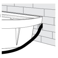
13 Before gluing black flexible PVC pipe verify the factory installed fittings are tight. Then glue the black flexible PVC pipe into the 45 degree elbow that is pre-installed.
