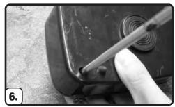
Re-install screws into compressor housing.
