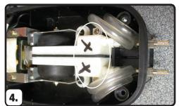
Install new diaphragm with air outlets to the bottom. Be sure "X's" are up as shown.
