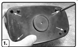
Unplug unit and remove the four screws from the bottom housing of the compressor.
