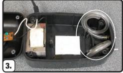
Remove the diaphragm from compressor leaving the air tubes. Inspect magnets and clean if needed.
