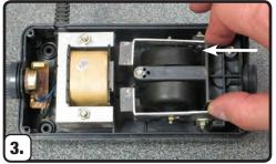
Remove the diaphragm from compressor. Carefully lift straight up to avoid damaging threaded posts.
