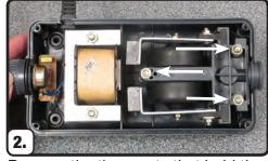
Remove the three nuts that hold the diaphragm to the base.
