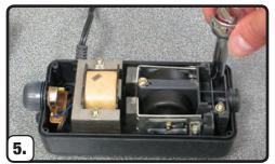
Install replacement diaphragm and re-install nuts.
