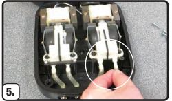
Match the air outlets to the air tubes and re-install screws.
