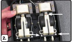
Remove the three screws that hold the diaphragm to the base.
