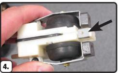
Locate metal bracket on back of repair kit and be sure it is up when installed.
