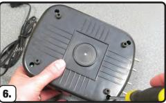
Re-install screws into compressor housing.
