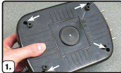
Unplug unit and remove the 4 screws from the bottom housing of the compressor.
