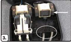
Remove the diaphragm from compressor leaving the air tubes. Inspect magnets and clean if needed.
