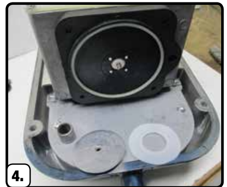
4. Unthread the 7mm nut and remove the metal retainer plate, note the orientation of metal plate for reassembly.
