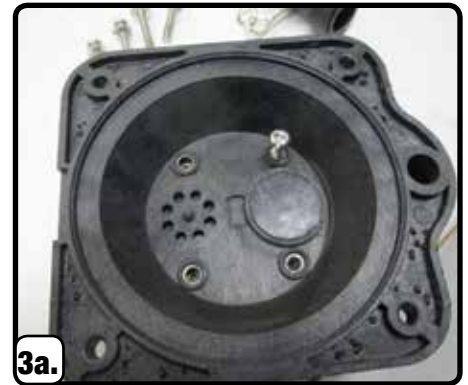
3a. To access flapper valves remove housing.
