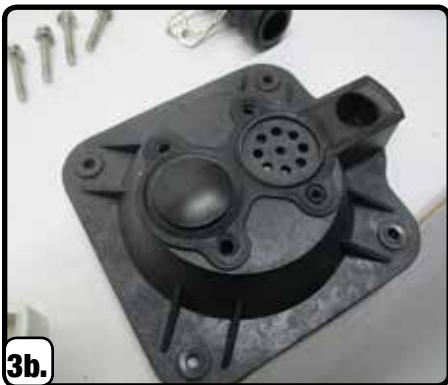
3b. Remove and replace black flapper valves, trim excess from tip of flapper valves.
