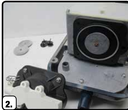
2. Remove the black air hose with the two spring clamps, unscrew the plastic assembly by removing the four screws.
