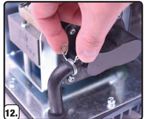
12. Reattach L-tube and secure with existing pinch clamp.
