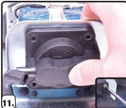
11. To install new diaphragm outlet cover, be sure to properly align holes and hold tightly while securing with screws. Gradually tighten screws around the assembly until evenly tight to unit.
