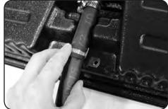
Fit padded hose clamp over tubing. (Use 17.5mm clamp for <sup>3</sup>/<sub>8</sub>" tubing) (Use 25.5mm clamp for <sup>1</sup>/<sub>2</sub>" tubing)
