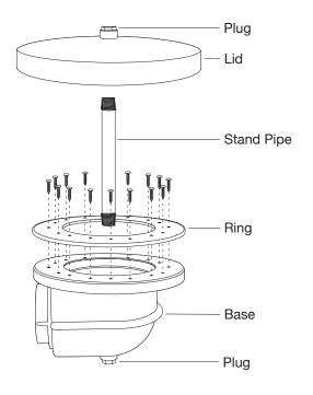
■ Drain base is installed under the liner, usually in the deepest part of the pond. Determine placement and excavate. Bottom drain and plumbing use a PVC 4" male adapter or reducing adapter to connect to PVC pipe (not included). Teflon tape threads of male adapter and tighten securely to prevent leaking.
