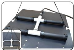
8. To install diffuser, loop a rope around 9. Once in place on the pond botthe plate and insert in supplied grooves. Lower the self-weighted diffuser assembly to the pond bottom using the rope to assist.
