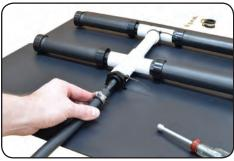
5. Slip hose clamp over the end of the tubing and push tubing onto the fitting.
